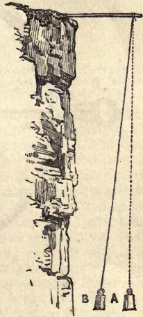
Fig. 12. The Schichallion Rocks. The dotted line and weight A represent the ordinary position of a plumb-line, whilst the line of the weight B indicates (of course, with some exaggeration) the attractive power of the mass of the rock drawing it from the perpendicular.
