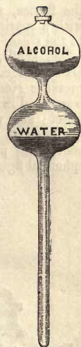
Fig. 383. Glass bulbs and tube to show the contraction in bulk of a mixture of alcohol and water.
