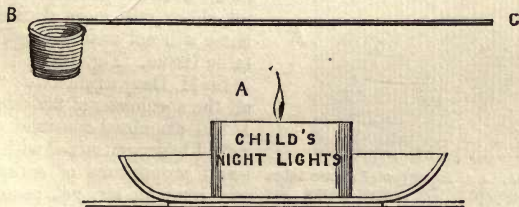
Fig. 360. A. Small flame from night light. B C. Large mass of cold copper wire open at both ends to place over flame, and by conduction of the heat to extinguish it.
