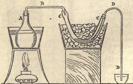
Fig. 156. A. The flask containing the phosphide of calcium and water, and placed in a water-bath heated to 140^{\circ} Fah. B. Bent tube conveying the gas to c c, the U-shaped tube, to which it is attached by india-rubber tubing. c c. The U-shaped tube, surrounded with a freezing mixture. D D. Bent tube, passing into a cup of water to prevent contact with air.
