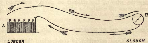
Fig. 210. A. The battery. B. The instrument. The arrows show the passage of the electricity to the single needle telegraph instrument by one wire, and the return current by the other.
