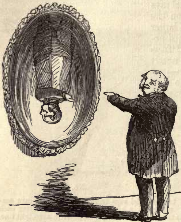
Fig. 273. A concave mirror, showing the appearance of the inverted and reflected image in the air.
