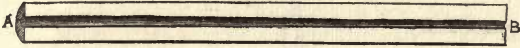
Fig. 348. A B. Magnified view of the bore of one of the thermometer tubes which are made by rapidly drawing out a hollow mass of hot glass whilst soft and ductile, consequently the bore must be conical, and larger at one end than the other.
