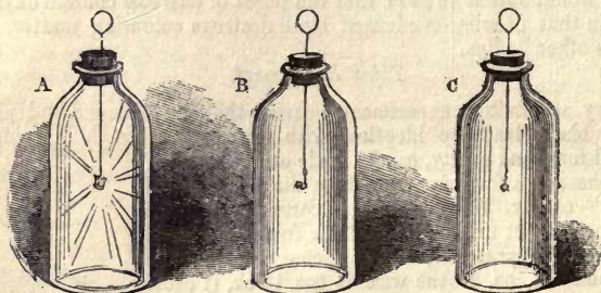
Fig. 146. A. Bottle containing bark charcoal. B. Ditto the plumbago or black lead. C. Ditto the diamond.
