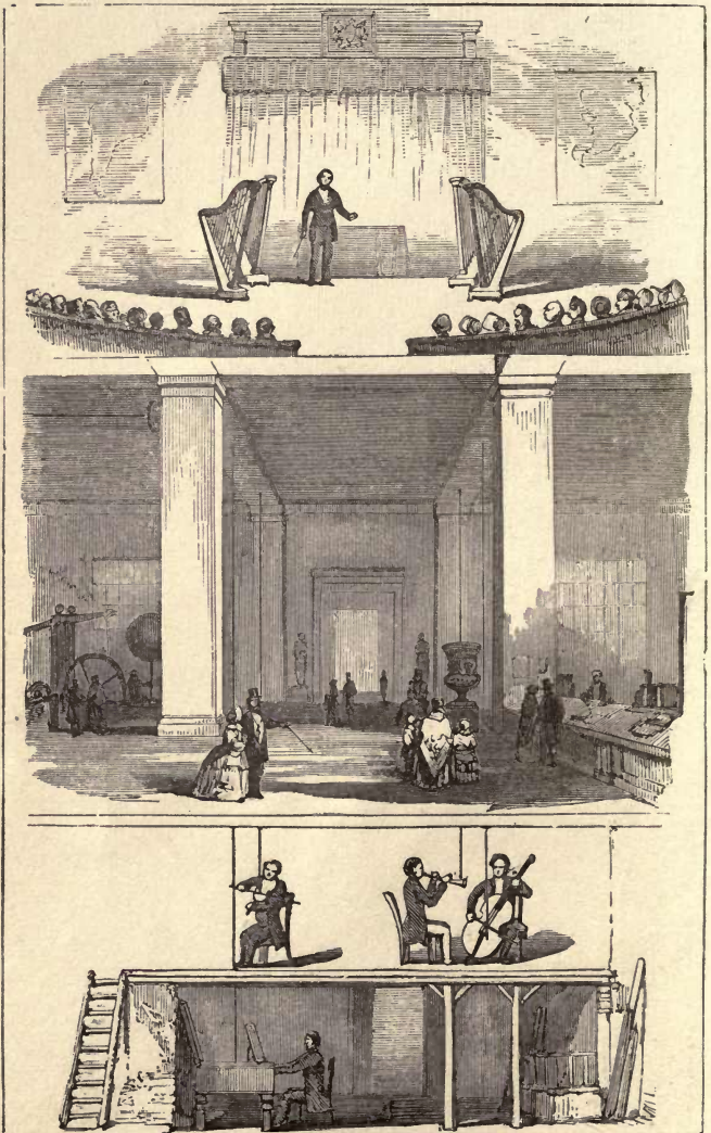
Wheatstone's telephonic concert at the Polytechnic, in which the sounds and vibrations pass inaudible through an intermediate hall, and are reproduced in the lecture-room unchanged in their qualities and intensities. Frontispiece.
