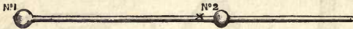
Fig. 349 a.—No. 1. First bulb. The intended length of the thermometer is shown at the little cross.—No. 2 is the second bulb placed above the cross.
