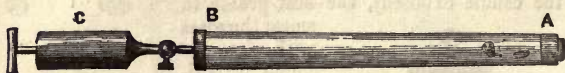
Fig. 19. A B. Glass tube containing a piece of gold and a feather, which are placed in at the large aperture A. C. Small hand-pump.
